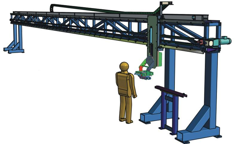
Test systems can include 4, 6, 8 or more transducers, arranged in any combination to detect longitudinal, transverse or lamination defects, using shear wave or longitudinal wave methods as appropriate. Choice of the number and arrangement of transducers is between Supplier and Customer, and it is often governed by code requirements.
