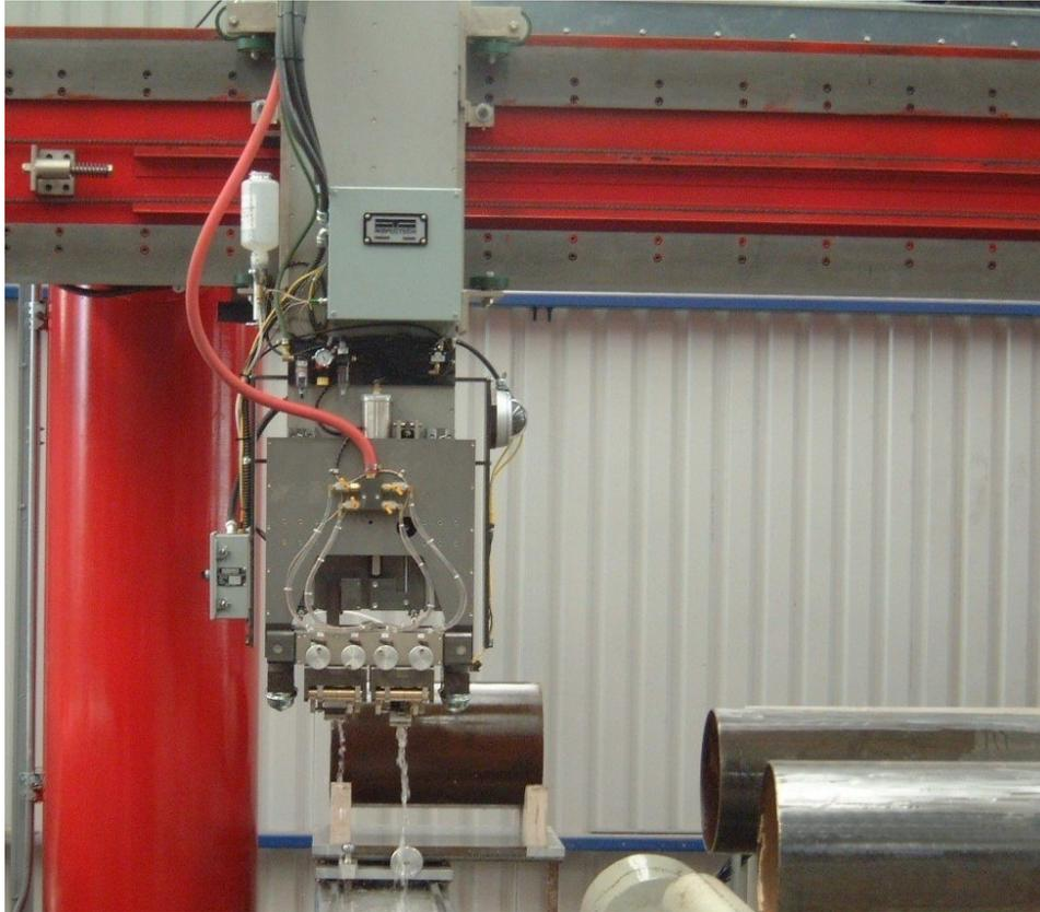
InspectTech<sup>®</sup> Off-Line Ultrasonic Test Systems are specially designed and configured to inspect the entire length of a weld seam in a tubular product. This form of testing is normally required for code compliances such as API and ISO. Testing is similar to InspectTech's On-Line Test System, but the test head is configured differently and more mechanization is required.
