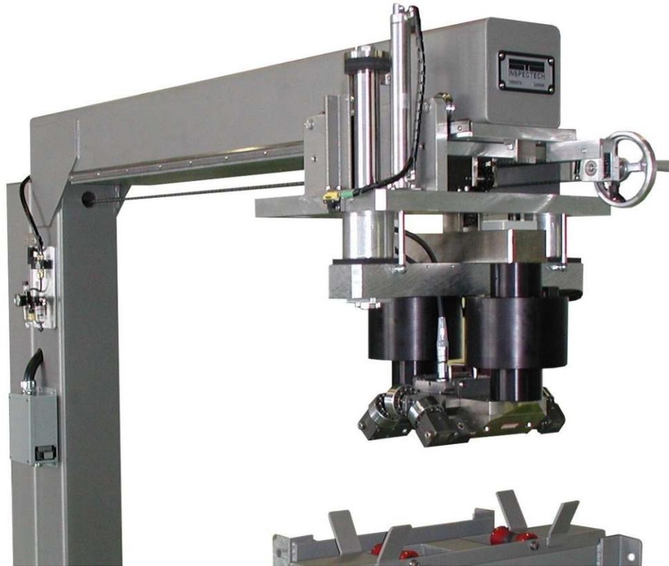
The Flux Leakage method of testing tubular goods has been used for many decades for full body inspection. Using this method to test weld seams in small diameter (12mm and up) tubes has, up to now, not been practical because of the difficulties in obtaining uniform magnetic fields with minimal pole piece spacing.
