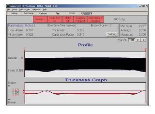
Typical operator screen showing the thickness and prof le of the weld zone.
